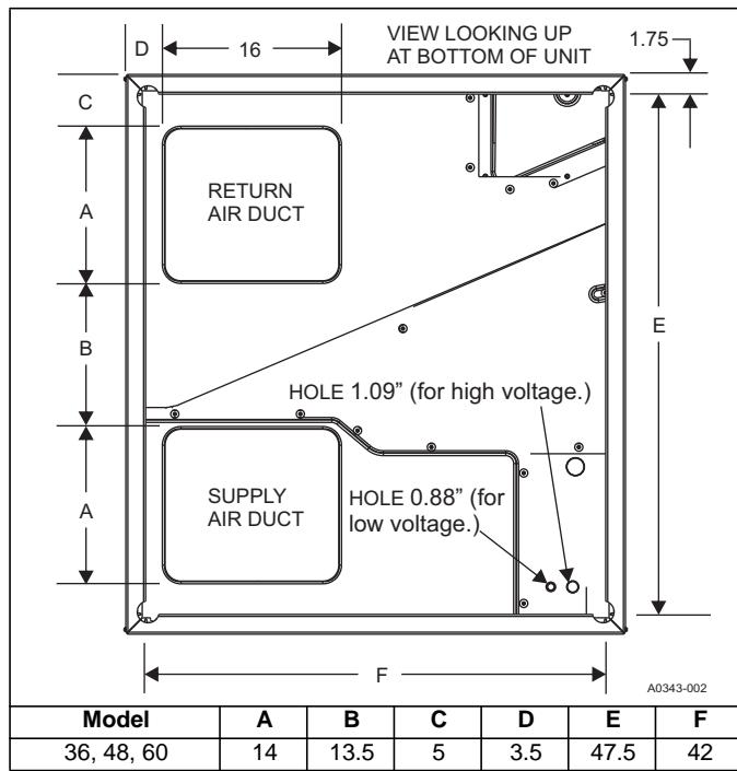
**REAR DUCT DIMENSIONS (in.)**
